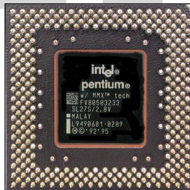
Figure 1.5 : Intel Pentium Microprocessor Chip
