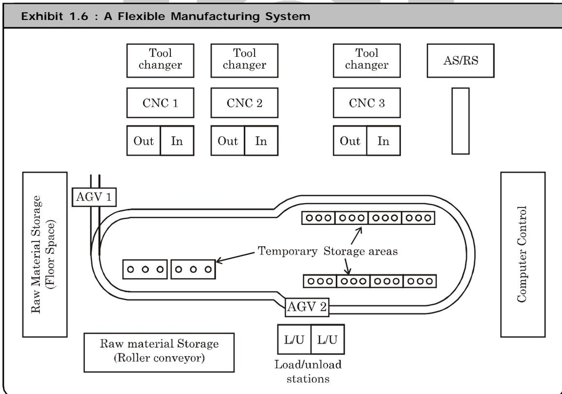
An FMS is a type of **flexible automation system** which builds on the programmable automation of NC and CNC machines. Materials are automatically handled and loaded and unloaded for machining operations. Programs and tooling setups can be quickly changed and production can be quickly switched over from one job to another with no loss of change over time.
